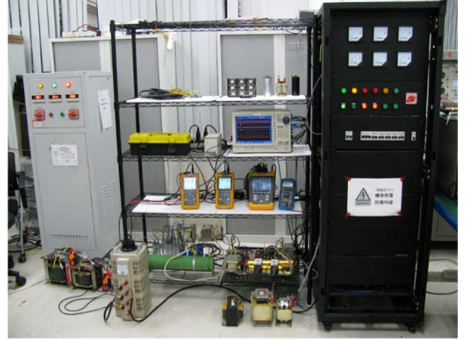
Fig. 20. Hardware appearance of laboratory-scaled hardware prototype of co-phase supply with railway HPQC.
